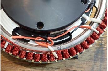
The controller is a generic cheap 350W module from china that has been removed from its case to fit inside the motor as the original one had been removed before I got it. To continue the budget theme I powered it from several used 36V Hoverboard batteries I had left over from a past project.
