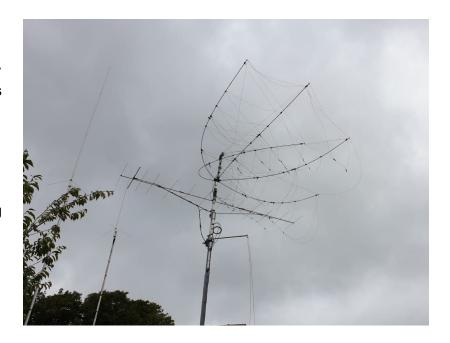
I have since been in conversion with Ant (MW0JZE) the manufacturer who was amazed the portable was even being used as a permanent antenna. A replacement spreader section has been ordered together with him providing me with some information regarding storm cords. The storm cords will stop the spreaders being pulled up over the top and will hopefully enable it to weather these sorts of storms. Time will tell.
