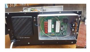
required. Not easy! In this amp a specially modified LDG auto ATU is employed to match the input requirements. This can be seen at the back of the amp in the photo. This ATU is automatically band switched by Rf sensing and it ensures a low input VSWR on all bands.
