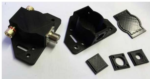
We did some tests last Friday at the club running 100 watts constant through the balun. I also used the balun with an inverted-v cut for the 20m band last weekend, and managed to work KG1E on 15watts. so all seems to be working well.
